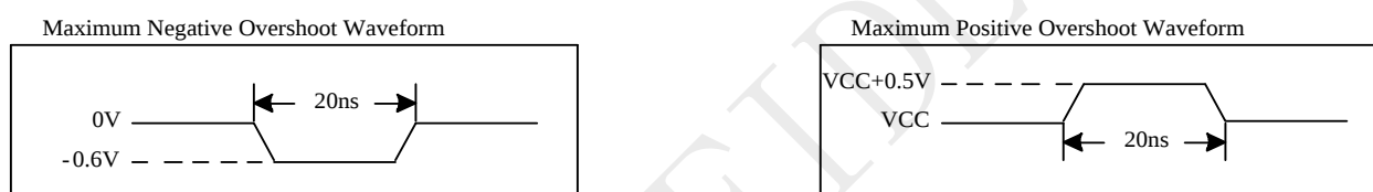
Figure 5-1 Maximum Overshoot Waveform
