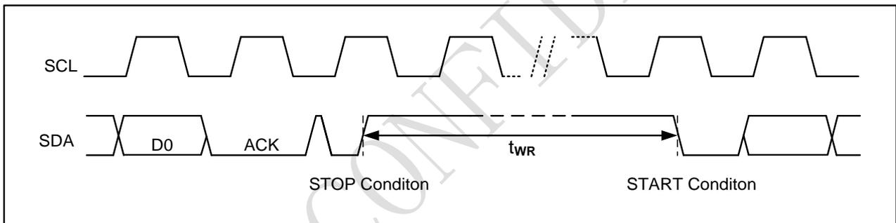
Note: [1] The write cycle time  $t_{WR}$  is the time from a valid stop condition of a write sequence to the end of the internal clear/write cycle.
